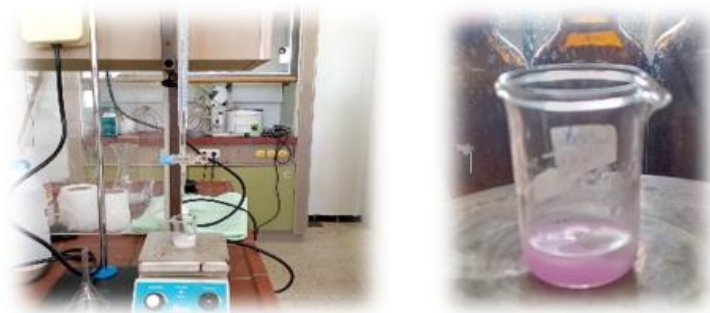
Figure 0.4: Standard test method for determination of acidity in essential oils by titration
