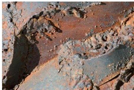
**Figure I-9:** corrosion-érosion
