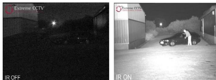
FIGURE 2.3 – Standard camera on left ; integrated Active-IR on right [27]
