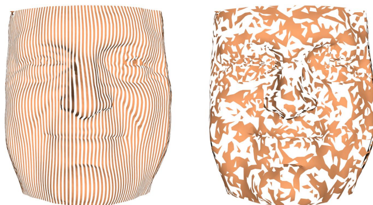
Figure 1.19: Generating triangle strips from a polygonal data set. On the left, the original laser range data is stripped; on the right, an unstructured mesh (after decimation) is stripped. [61]
