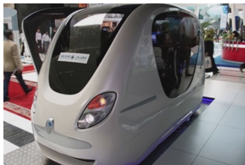
Figure 16: The PRT vehicle developed for the Masdar eco-city project in Abu Dhabi. source: courtesy of ‘2getthere’
