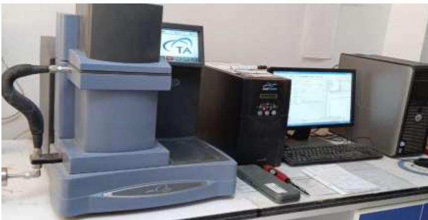
Figure III.16 : Machine DMA de marque DMA Q 80
