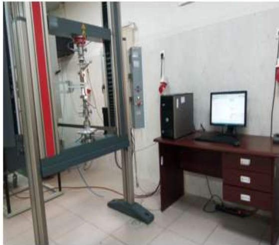
Figure III.8 : Machine de traction de type Zwick/Roell
