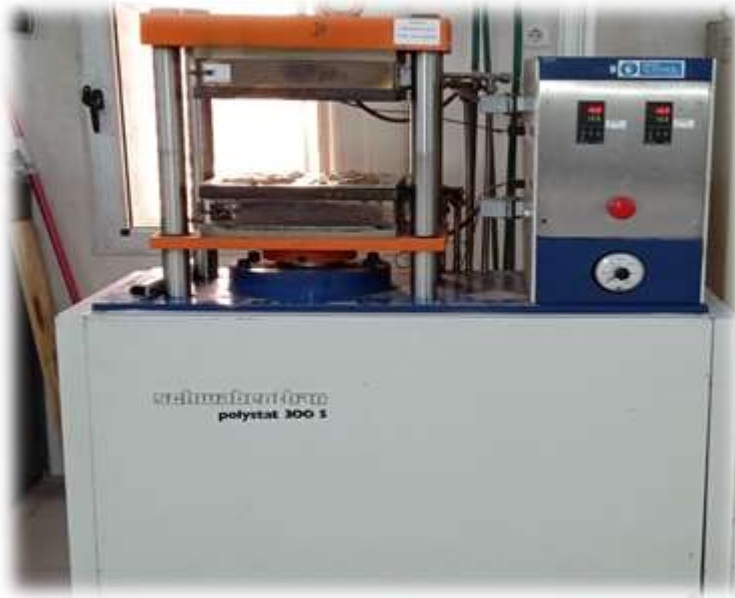
Figure III.6 : Machine de moulage hydraulique Schwabenthan polystat 300 S
