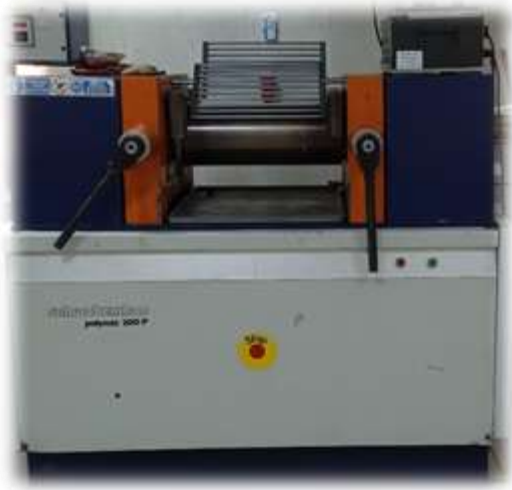
Figure III.4 : Machine de calandrage Schwabenthan poly mix 200
