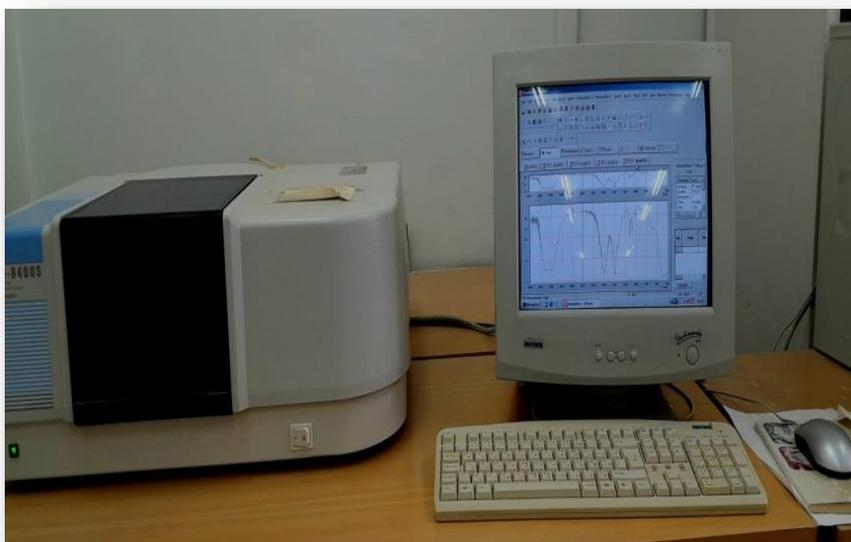
**Figure II.18:** Thermo Scientific FTIR instrument (Nicolet 8400s).
