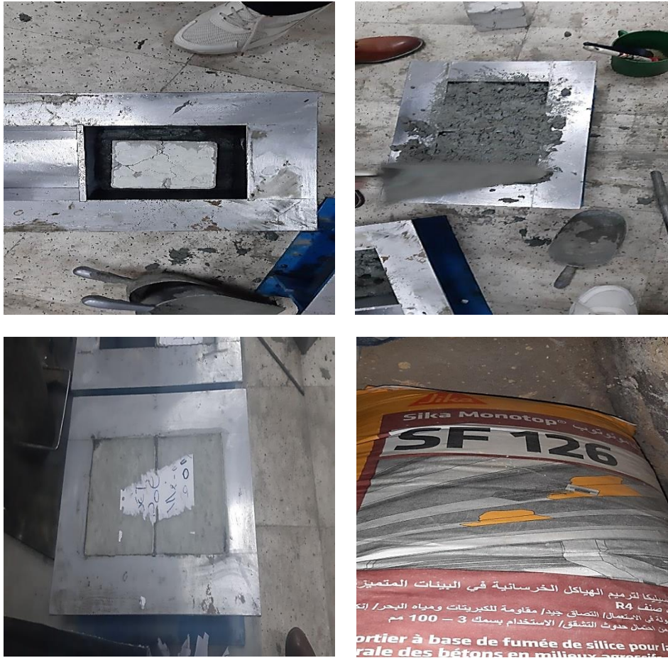
Figure III. 20 Repair procedures for specimens heated to 750°C with both our prepared repair concrete and a commercially available repair mortar.
