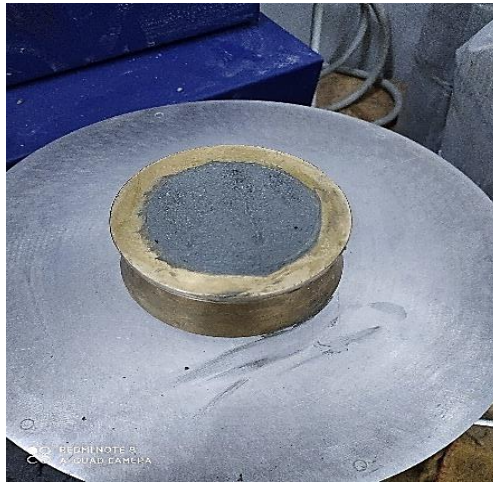
Figure III. 7 The flow test of polymer mortars.
