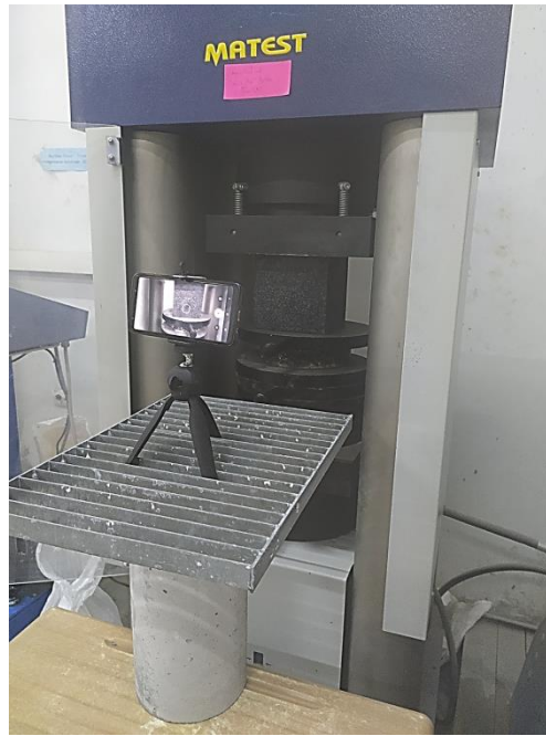
Figure III. 23 Device for image correlation.
