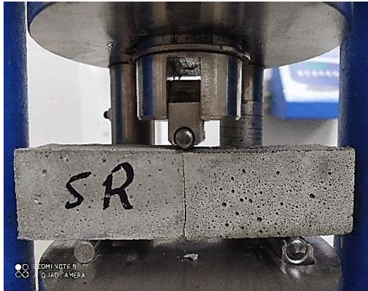
Figure IV. 24 Two-component mortar after rupture.
