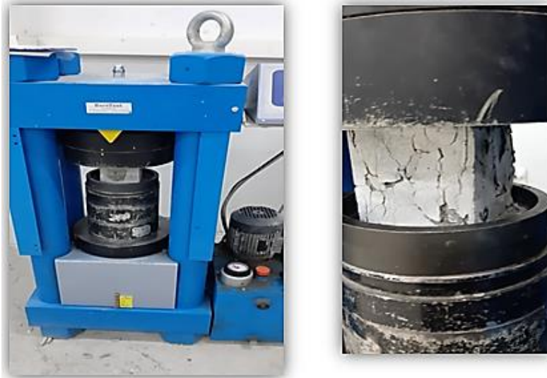
Figure III. 17 Apparatus for measuring the compressive strength of heated concrete.
