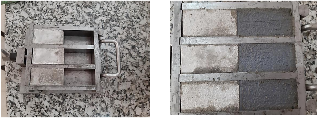
Figure III. 5 Preparation of substrate mortar and polymer mortar test specimens for adhesion testing.
