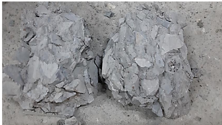
Figure IV. 28 Internal damage of specimens following the 750°C heating-cooling cycle.
