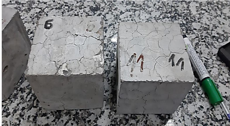
Figure IV. 27 Concrete specimens after the heating-cooling cycle to 750°C.
