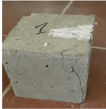
Figure IV. 30 Photo of test specimens repaired after crushing.
