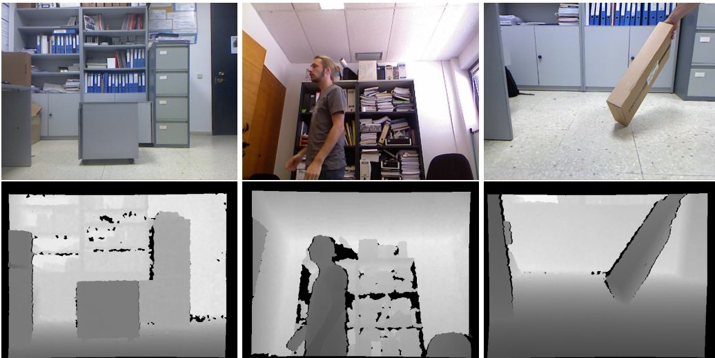
Figure 3.5: Some frame samples from SBM-RGBD Dataset, to illustrate the challenging categories. From left to right, ColorCamouflage , DepthCamouflage , and Shadows
