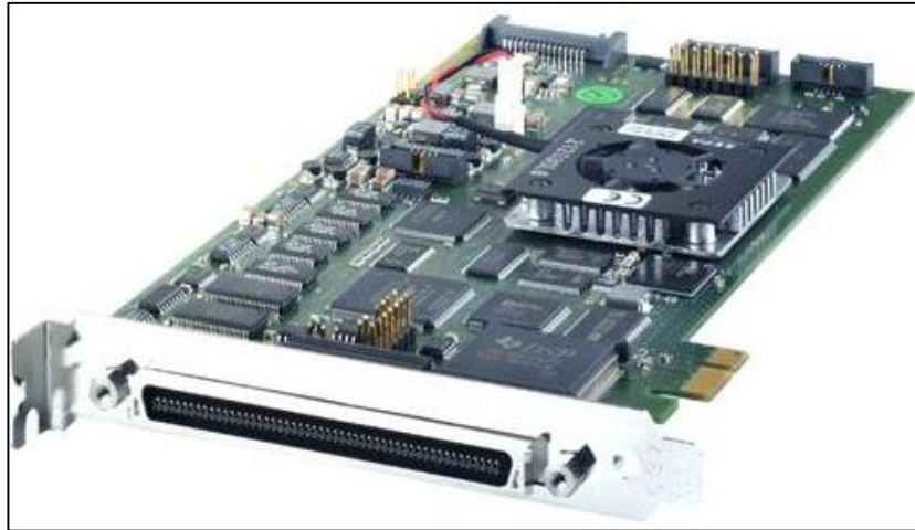
Figure A.3. dSpace DS1104 control board.
