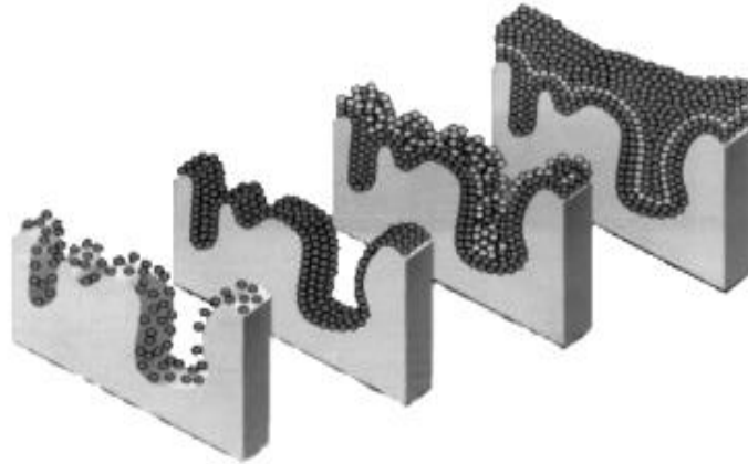
Figure I. 9: Representation of the adsorption of the adsorbent on the surface of the adsorbent (Arias, M et al., 2002)
