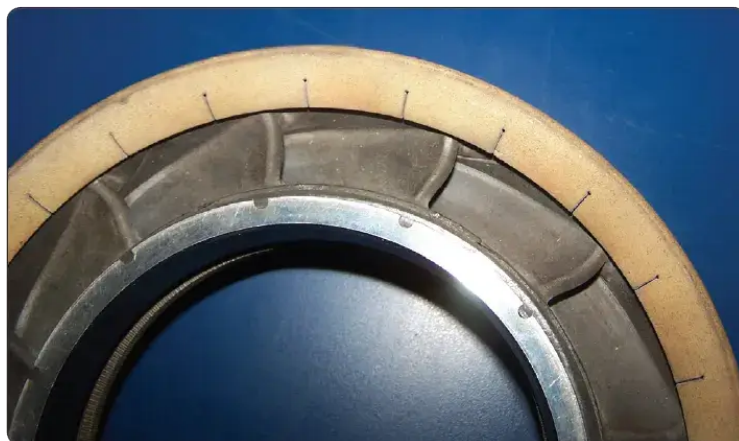
Figure I.4: Turbine inlet guide vanes (TIGVs) [6].
