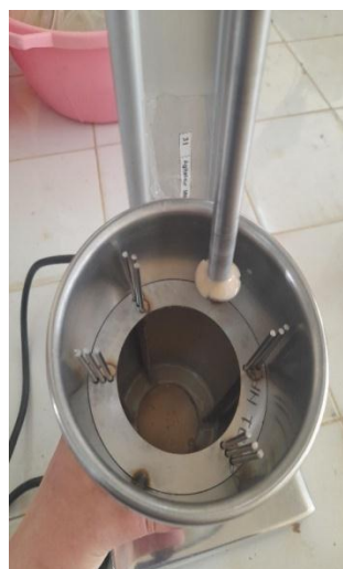
Figure 3.6 Agitator used to obtain homogenous blend for experiments.
