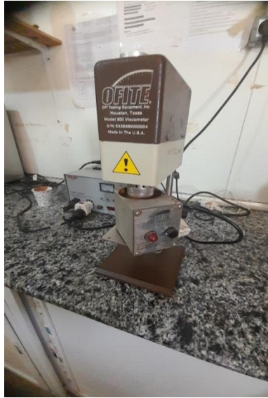
Figure 2.5 Rheometer Fann 35 used in laboratory construction site HASSI MSD
