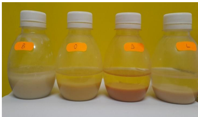
Figure 3.9 Different swelling capacities according to sedimentation volume for water -clay suspensions.
