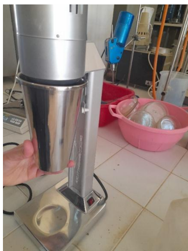
Figure 3.6 Agitator used to obtain homogenous blend for experiments.
