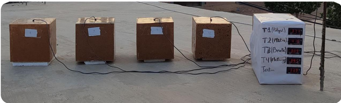
Fig.II.14. Performance thermique des structures Sandwich.
