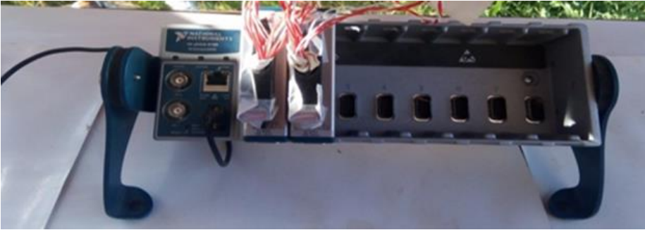
Figure II.8 NI Compact DAQ-9188 Ethernet 8-Slot chassis with 02 modules which supports 04-wire PT-100 Type temperature sensors.
