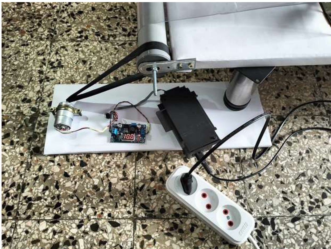
Figure 02: The power source (power supply, speed controller, motor)
