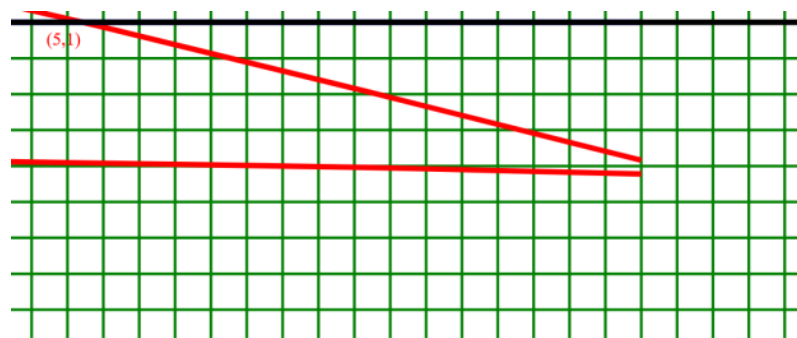
Figure II.11: Zoom in the trailing edge of the USA 35B [5].
