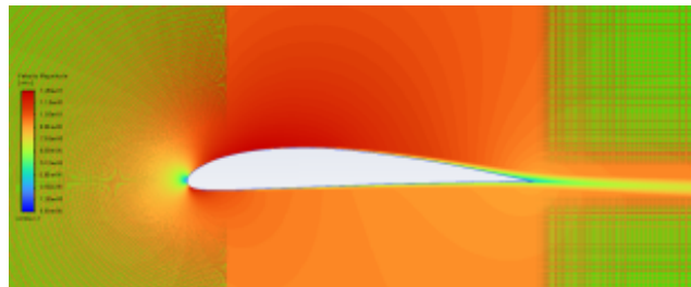
Figure III.4: The contour plots of velocity distribution at 0°
