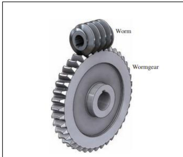
Figure I. 7 : Worm and worm gear with a single threaded worm[1].
