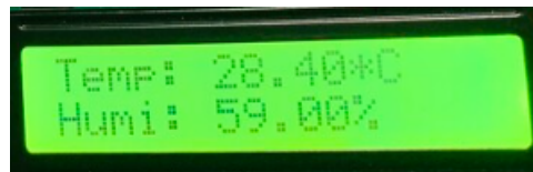
Figure 5.16: Result of DHT11 Sensor
