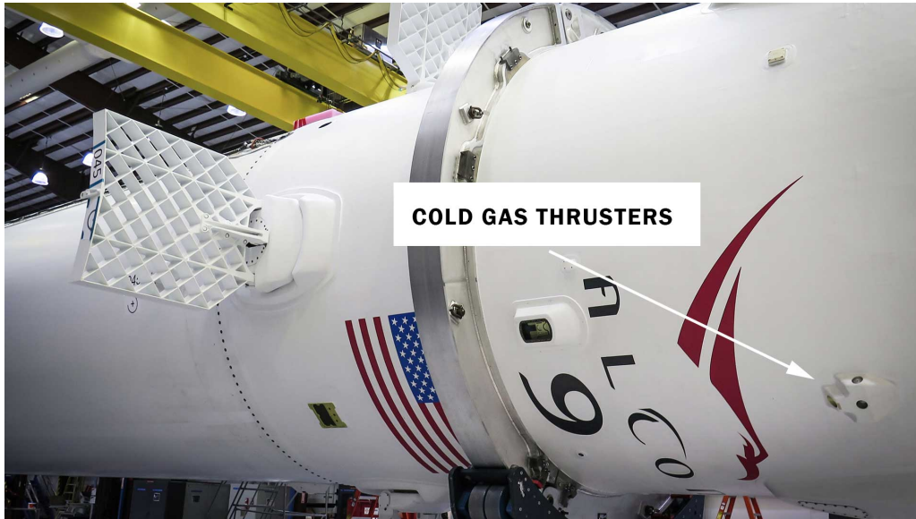
Figure 2.5: CGT On A Falcon 9 Rocket
