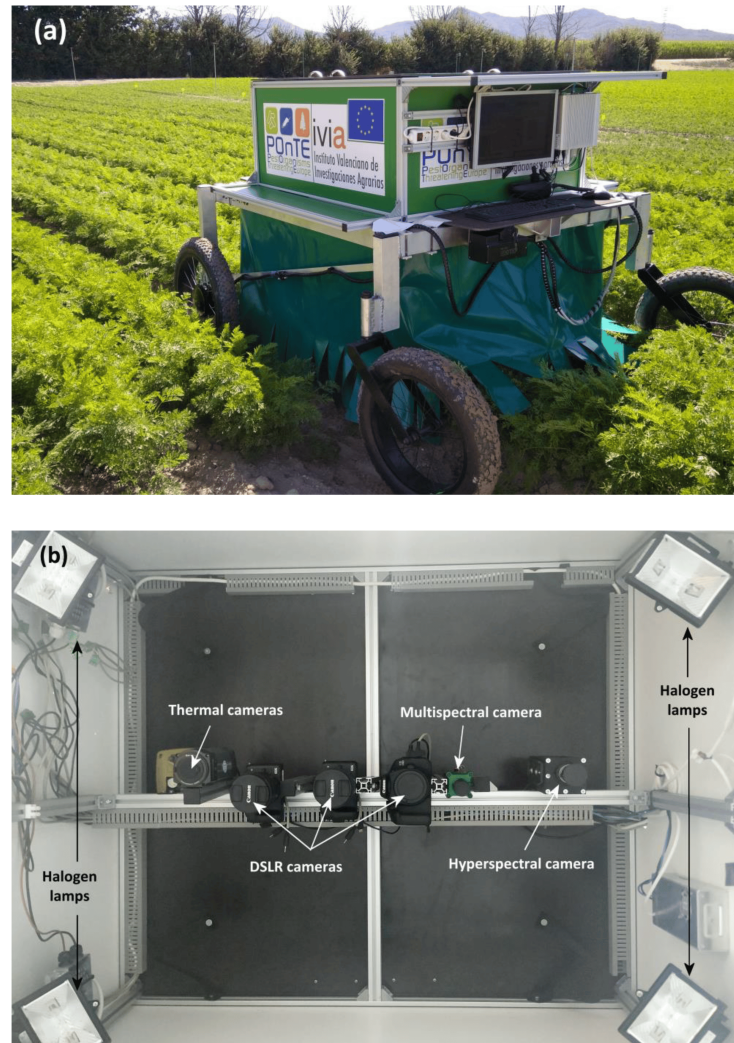
FIGURE 1.1: A remotely-driven RobHortic operating in a carrot field. (a) the external appearance of the robot. (b): inside from the plant point of view [1]
