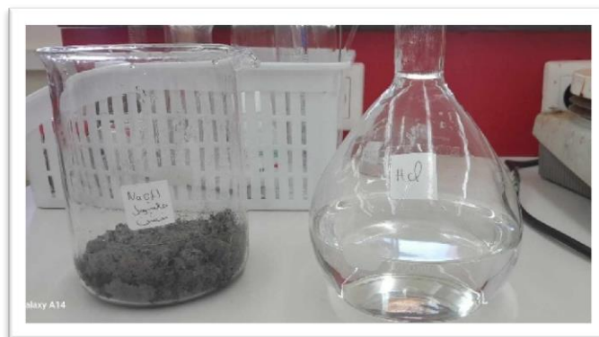
Figure II.10: Activated carbon washed with HCl and water with pH measurement.
