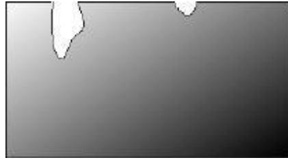
Fig I.3: Pitting corrosion of metal [16]
