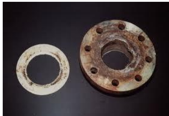
Fig I.6: Crevice corrosion of metal
