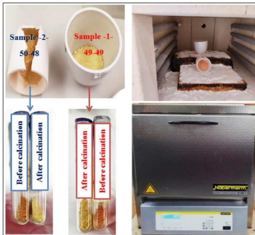
Figure II.13: The furnace used in the calcination process and the samples before and after calcination.
