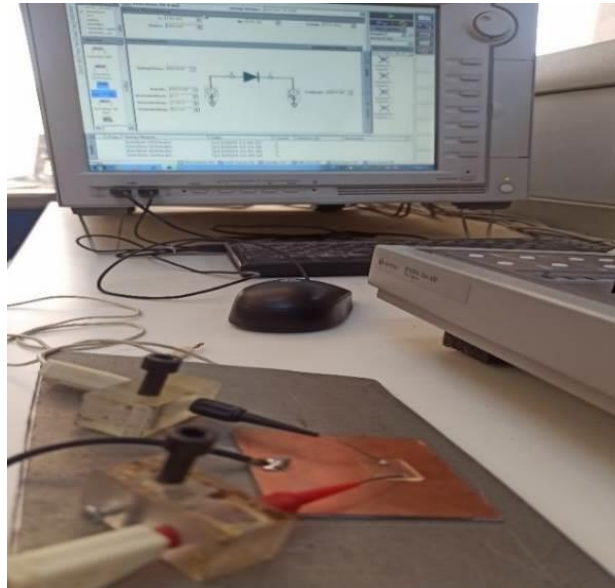
Figure II-20: B 1500 A Semiconductor Device Analyzes the I-V characteristics of Diode.
