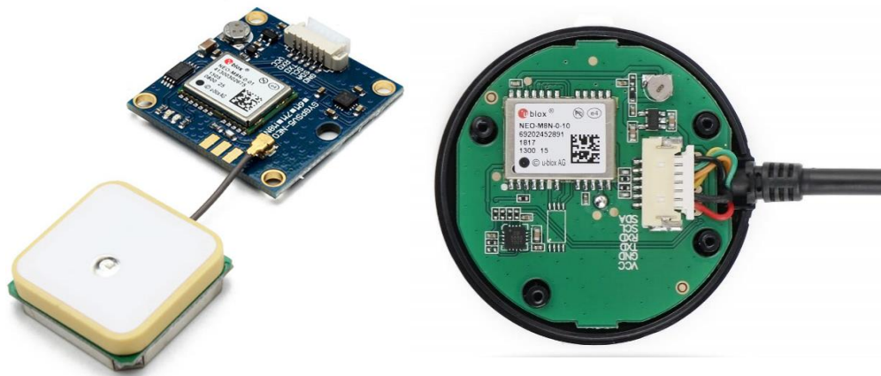
Figure 5.19: GPS for Positioning Measurement (U-Box GY-NEO-8M)
