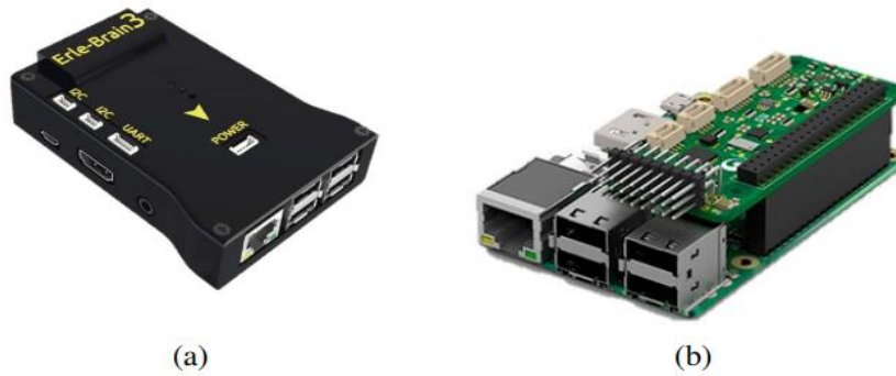
Figure 2.19: Open-source autopilot flight controller (a) Erle-Brain 3 (b) PXFmini Raspberry Pi family
