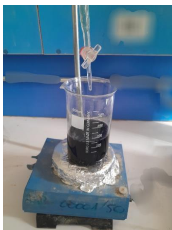
Photo 10: methode de Walkley et Black (photo original)
