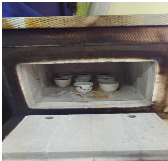
Photo 11 : methode de calcinations (photo original)
