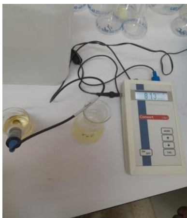
Photo8: Determination de pH ( photo original)
