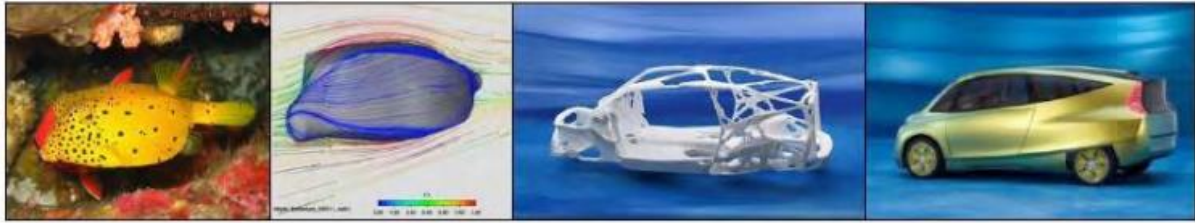
Figure 40: DaimlerChrysler bionic car inspired by the box fish and tree growth patterns. (Source: Pedersen Zari, M. 2007).
