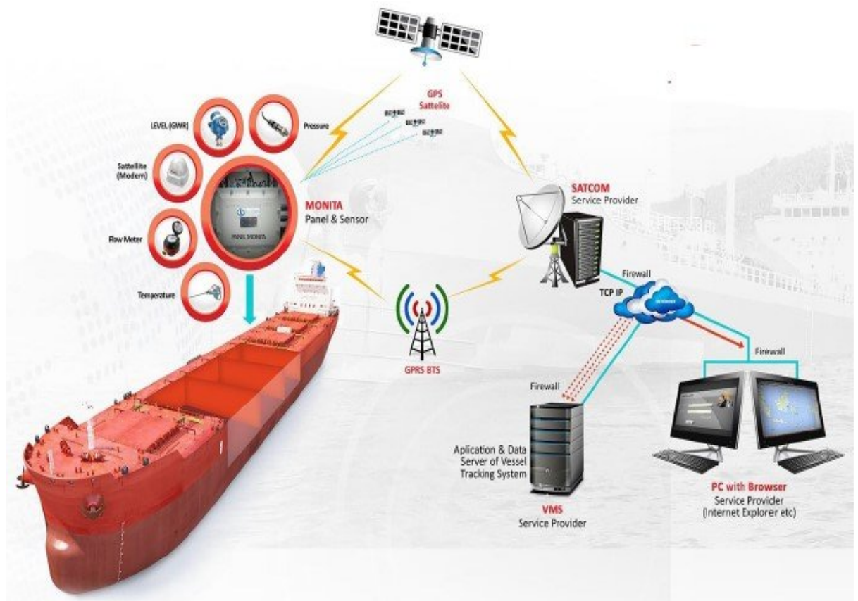
Figure 9 Diagram of a typical Vessel Monitoring System (Susanto, H., & Wibisono, G., 2019)
