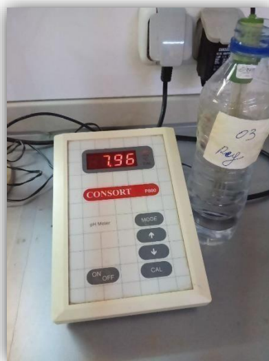
Figure III.8. pH meter used in the tests.
