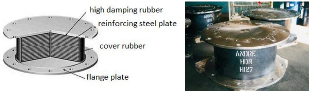
Figure I.3: construction of high damping rubber bearing[4]
