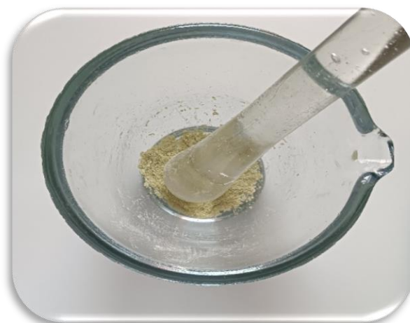
Figure II.20: Regrinding of the powder in a glass mortar
