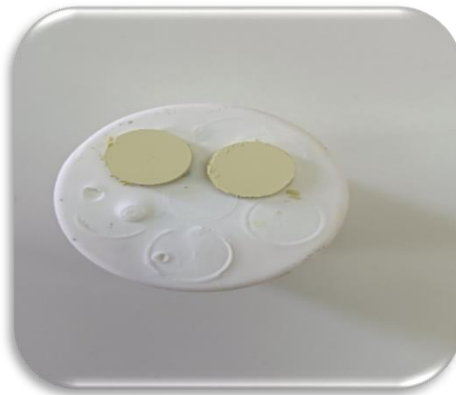
Figure II.22: Pellets before sintering
