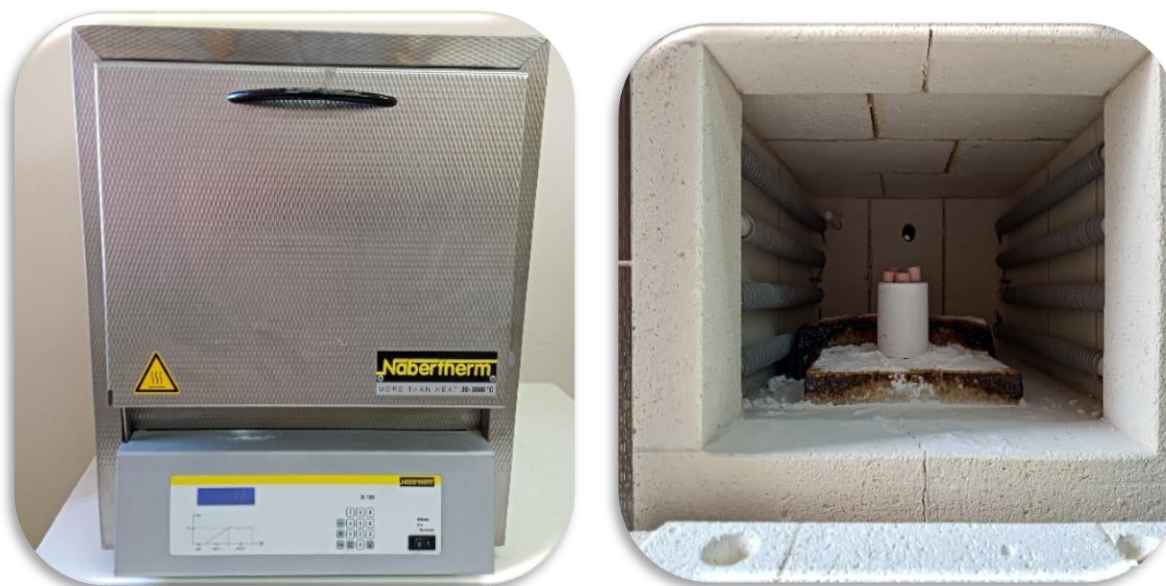
Figure II.13: Programmable furnace for calcination
