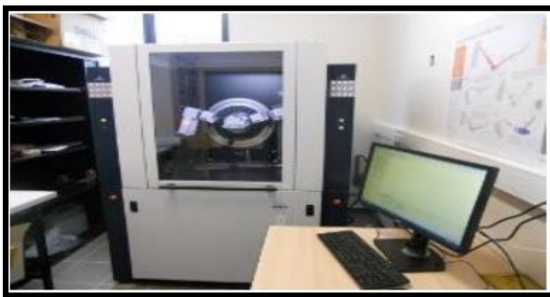
Figure II.3 : diffractomètre de type D8 Advance Bruker [4].
