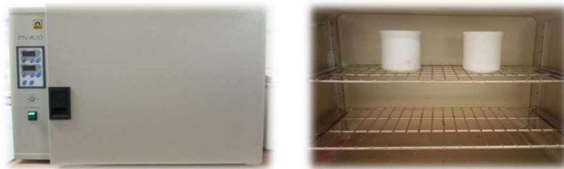
Figure III.2. Oven used for drying the powder mixture.
