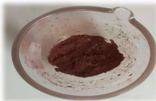
Figure III.3. Powder after grinding in a glass mortar.
