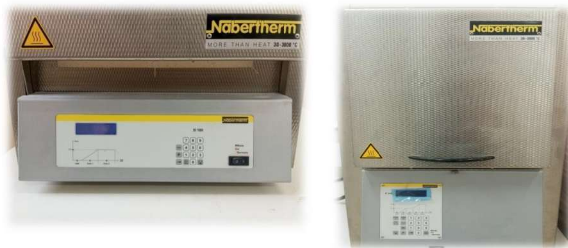
Figure II.1. Programmable Furnace used for heat treatment.
