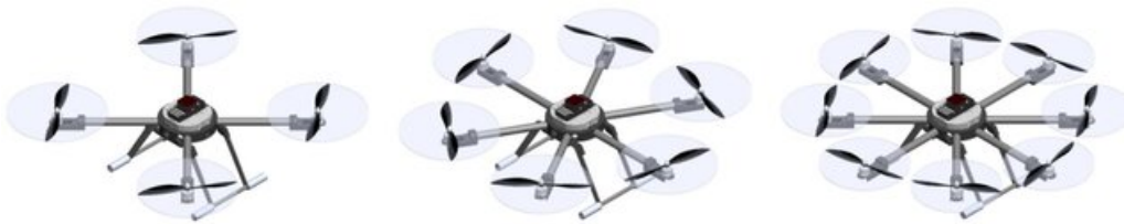
Figure 1.7. Multirotor drone structure [44].
