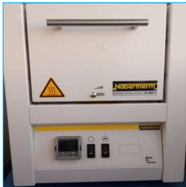
Figure III-3: Furnace for Heat Treatment.
