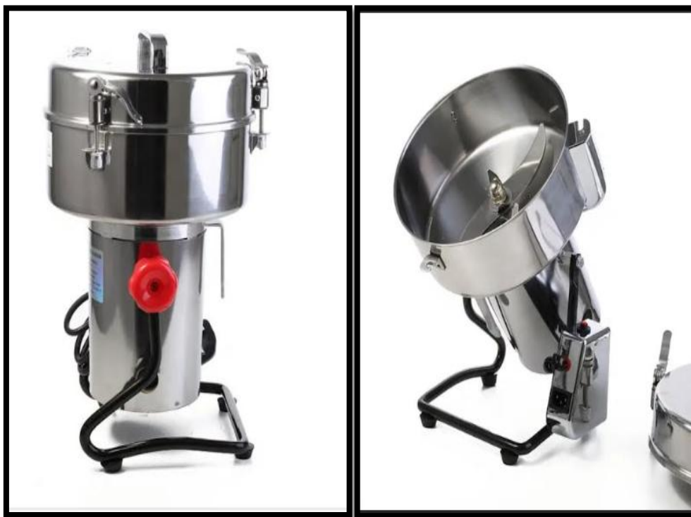
Figure II .7 Apparatus for the grinding process (RRH-3000A).
