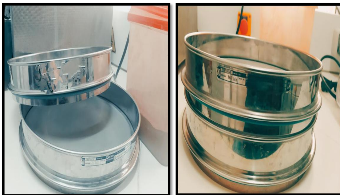
Figure II.8 A picture of the sieving process when 160 \mu\text{m} .
