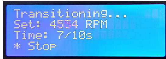
Figure 5.11: Transition phase execution screen
