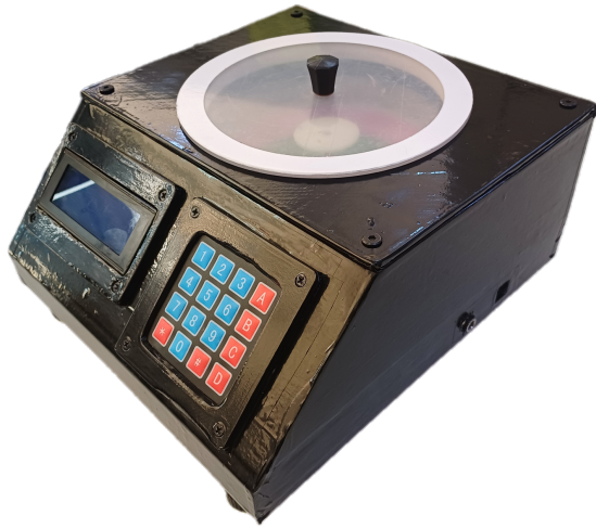
(a) Our homemade spin coater ($400).
