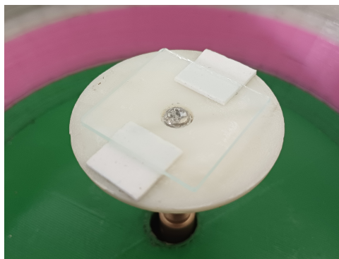
Figure 4.1: Substrate attached to spinning plate with double-sided tape
