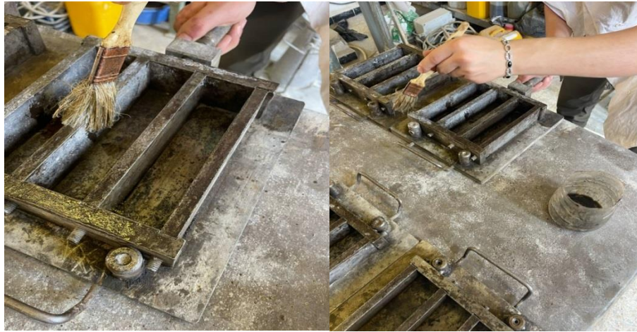
Figure II.18 : Lubrification des moules
