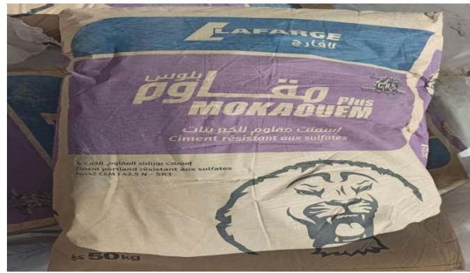
Figure 4. 1: Ciment utilisé CEM I 42.5 N – SR3
