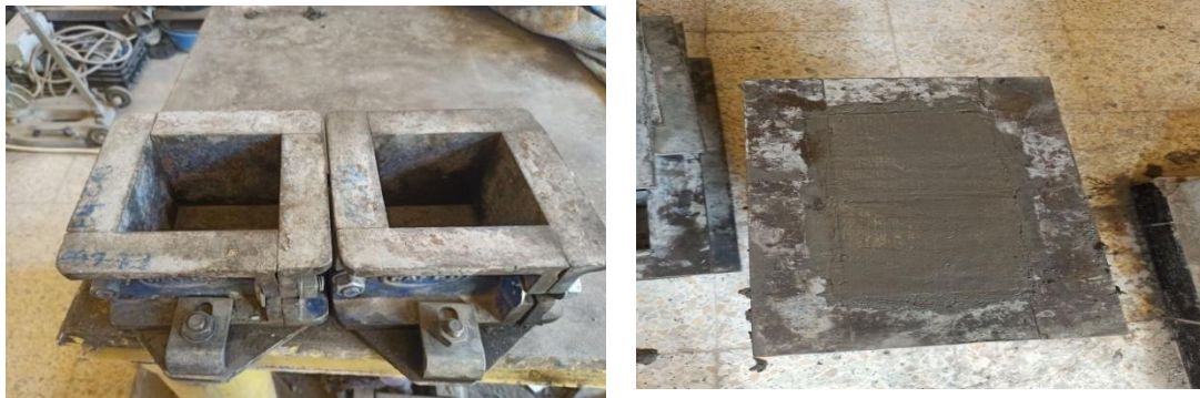
Figure 4. 20: Les moules cubiques ( 10 \times 10 \times 10 ) \text{cm}^3 .
