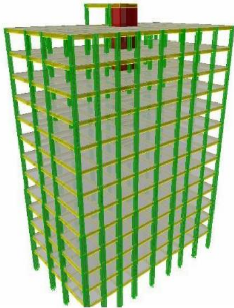
Figure 3.17 3D rendering view of building with fixed base in ETABS
