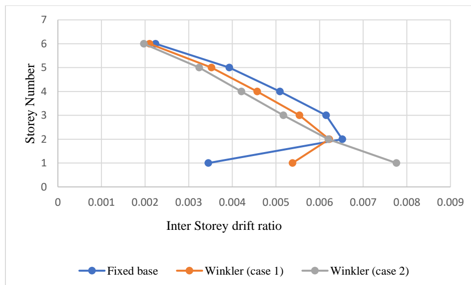
Figure 5.27 Inter-storey drift ratio vs Storey Number
