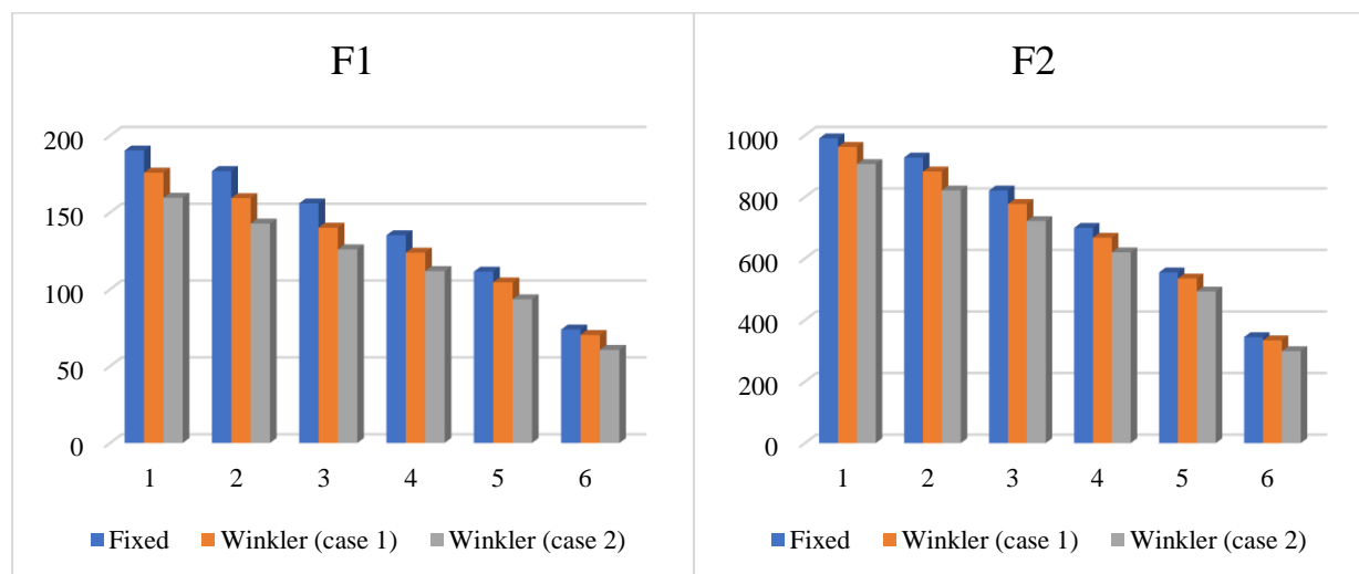
Figure 5.22 Shear Force Distribution in Y Direction for Different Support Conditions
