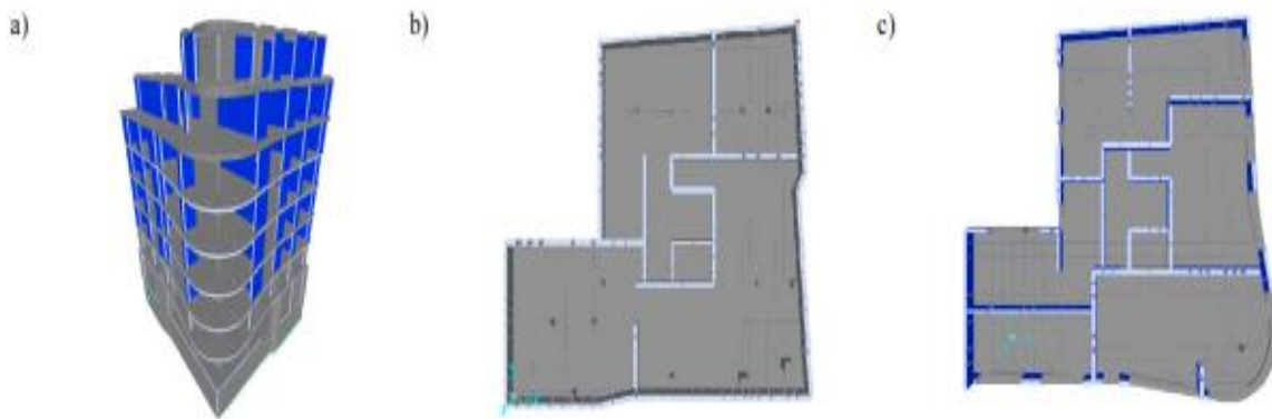
Figure 3.51 Perspective views of example building. Grey: concrete, blue: masonry. a) full model. b) plan view of foundation. c) plan view of 3rd residential floor
