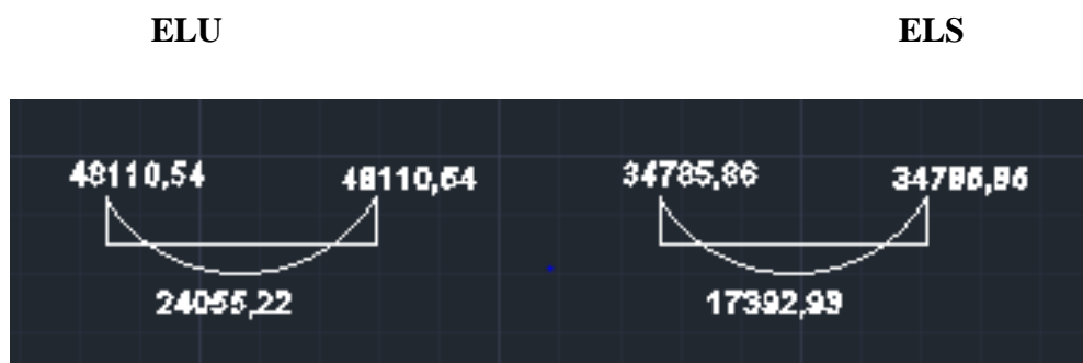
Figure III.10. Diagramme de moment.
