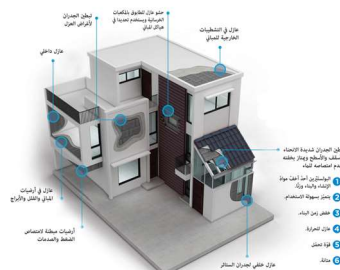
Figure 61: Techniques for improving thermal insulation in buildings
