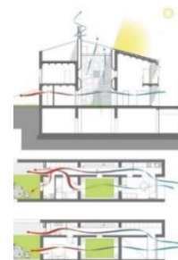
Figure 30: Longitudinal and cross section to illustrate Cross Ventilation
