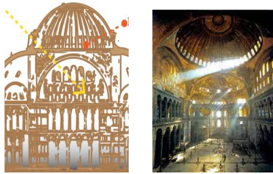
Figure I. 5 St. Sophia in Constantinople A.D. 532 - 537 now present-day Turkey with a ring of 40 windows making dome to appear to float and the pendentive allowed support of the dome at four points over a rectangular space
