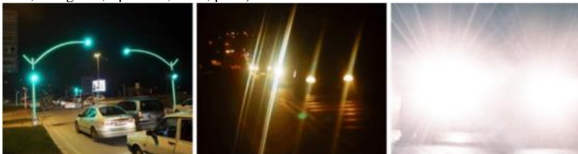
Figure I.15 Examples of three main types of glares -(a) discomfort glare; (b) disability glare; (c) dazzling or blinding glare
