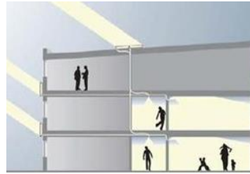
Figure 14 Fibre optics lighting technology (Zarewa et al., 2023)
