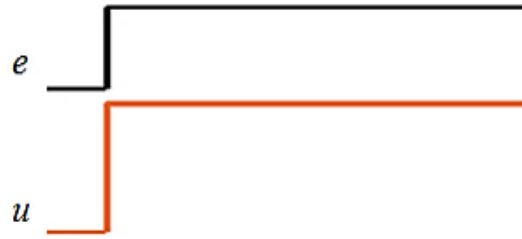
Figure 1.10 : Action proportionnelle P [2]
