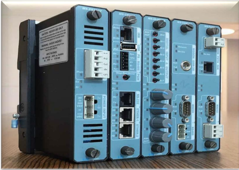
Figure 3.18. RTU (Remote Terminal Unit) [46]
