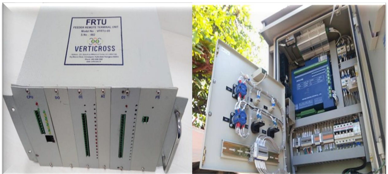
Figure 3.13. FRTU (Feeder Remote Terminal Unit) [40]
