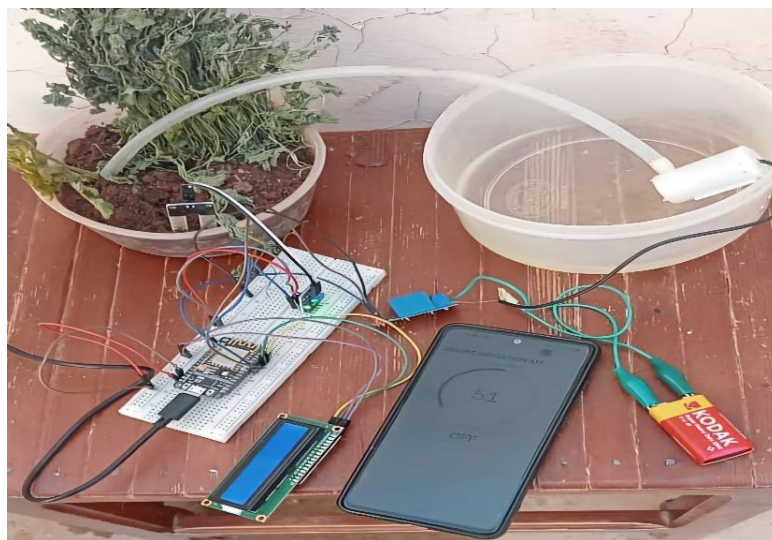
Figure.III.27: Test Project in Wet Soil
