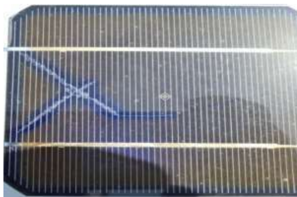
Figure III.5: Fissuration sur la surface de la cellule
