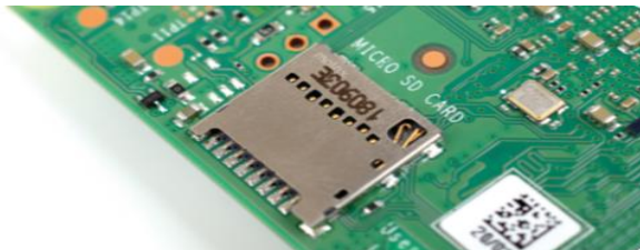
Figure II. 6: Support pour carte mémoire microSD [34].
