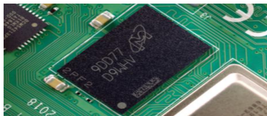
Figure II. 3 : La mémoire vive (RAM) du Raspberry Pi [34].
